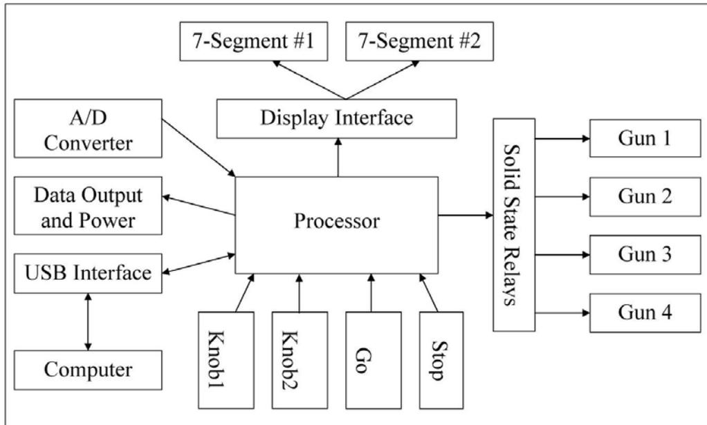
**Figure 1: Functional block diagram of the dynamic roadway marking system.**
