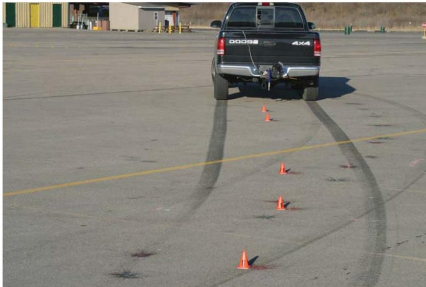
**Figure 5: Typical road evidence and paint marks from a test run. The different color paint balls signify the front or rear of the marker.**
