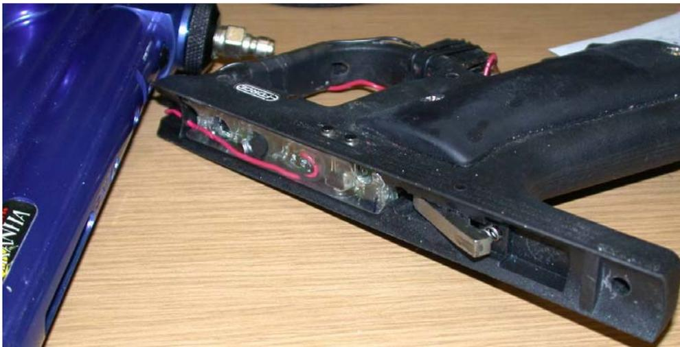
**Figure 3: Modifications to an off the shelf electronic paint ball marker. The mechanical micro switch is bypassed with a remote solid state relay.**
