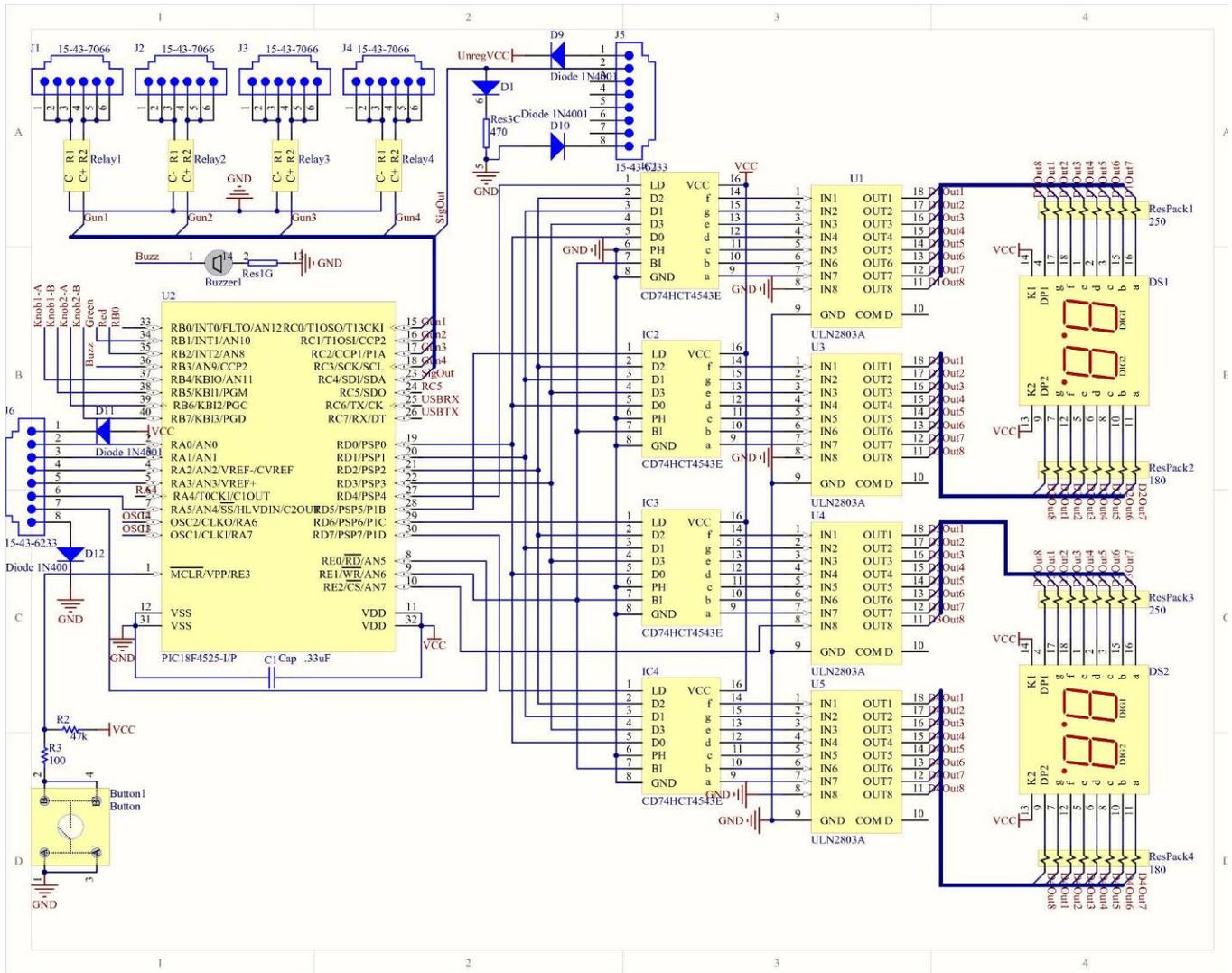
Figure 7: Schematic of the controller (page 1 of 2).
