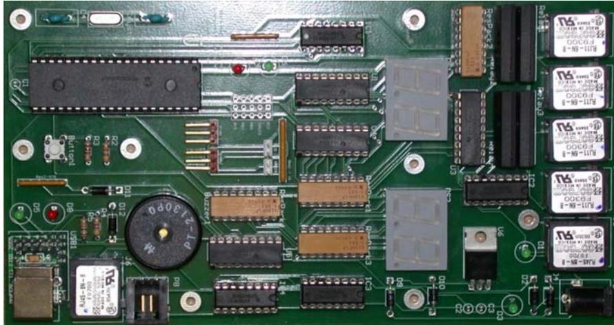
**Figure 2: A photograph of the actual implementation of the controller for the DRMS.**
