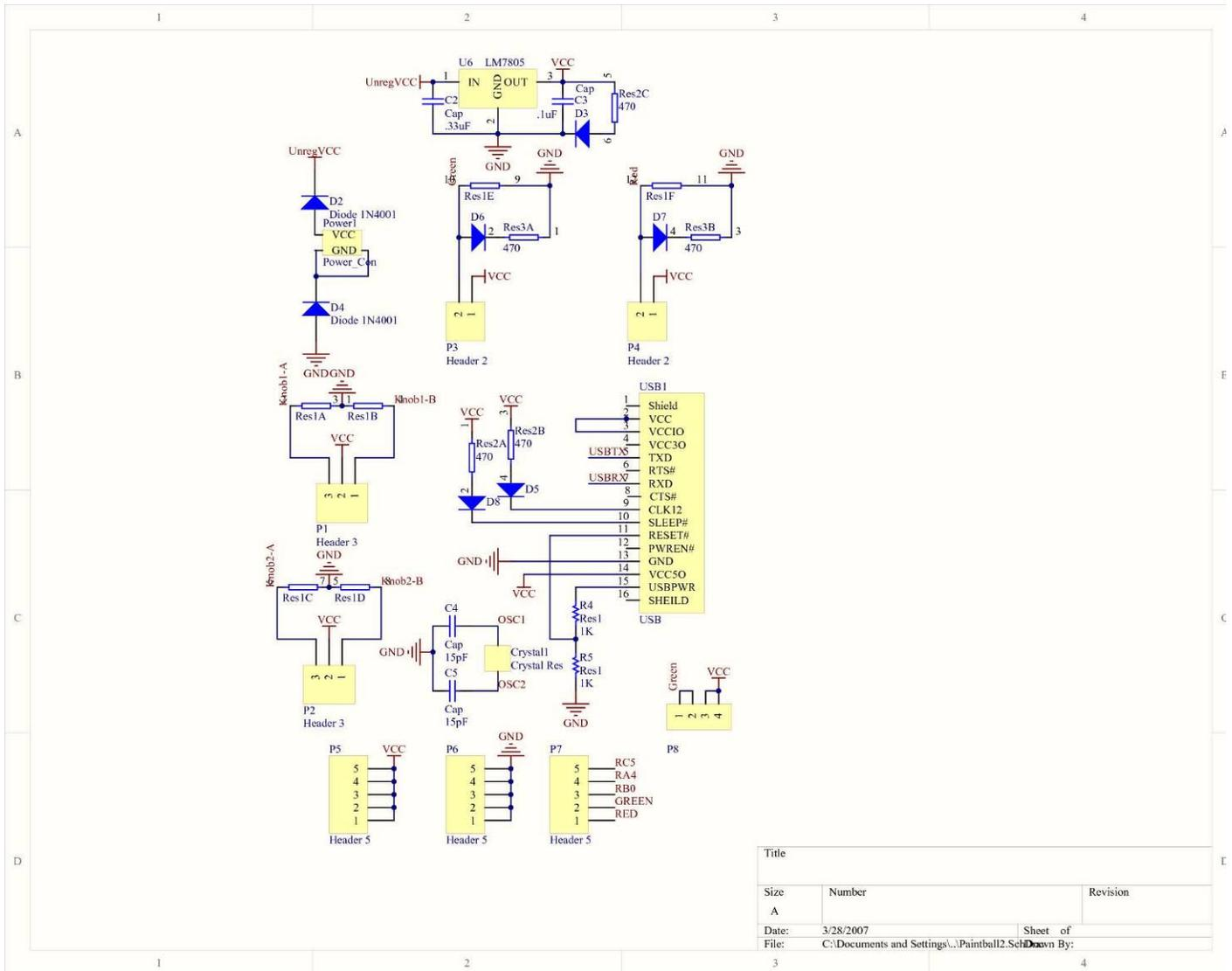
Figure 8: Schematic of the controller (page 2 of 2)
