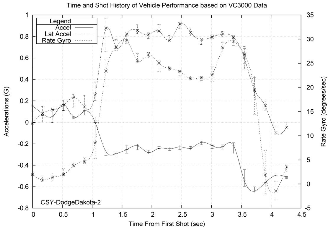
**Figure 6: An example plot of vehicle motion with points (with uncertainty) marked when paintballs were fired. The acceleration scale is on the left and the yaw rate scale is on the right.**
